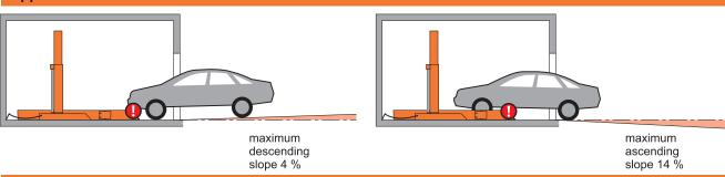
The illustrated maximum approach angels must not be exceeded. Incorrect approach angles will cause serious maneuvering & positioning problems on the parking system for which the local agency of the KLAUS Multiparking accepts no responsibility.
