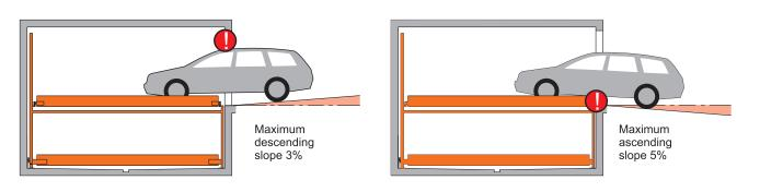
The illustrated maximum approach angles must not be exceeded. Incorrect approach angles will cause serious maneuvering & positioning problems on the parking system for which the local agency of KLAUS Multiparking accepts no responsibility.
