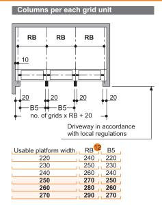
End parking spaces are generally more difficult to drive into. Therefore, we recommend our wider platforms for end parking spaces. Parking larger vehicles on standard width platforms may make getting into and out of the vehicle difficult. This depends on the type of the vehicle, approach and above all, on the driver's skill.
