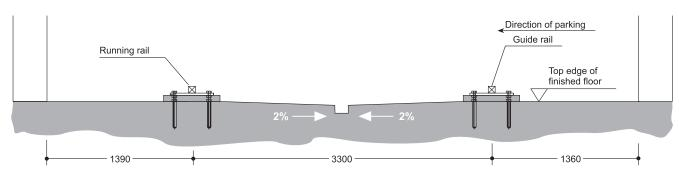
Tolerances for the evenness of the carriageway must be strictly complied with in accordance with DIN (= German Industrial Standard) No. 18202, chart 3, line 3.
