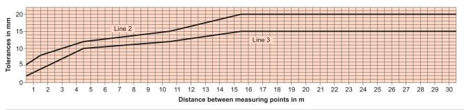
Intermediate values are to be taken out of the diagram and must be rounded-off to mm.
